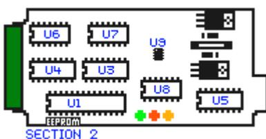
At this point, the WBo2 unit should be fully assembled with all discrete components and IC sockets, but no ICs should be loaded at this stage, except the DAC7612 (it comes pre-soldered to the PCB) and the 3 terminal 7058 voltage
