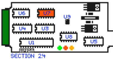
Install the **LMC6484** in position **U7** – note, it may be convenient to remove it later.
