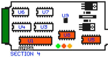
Power down the unit. Install **LMC6484** at **U8** (the right of the CPU). Power on unit. Note: **SVout** is available at **TP5** as well as **U8p9** and at **Y1p1**, which is the RJ45 connector at the right of the PCB. **p1** is at the bottom of **Y1** (PCB view) or left (connector view). Ensure the **TP5** signal is routed to the **Y1p1** output too.
